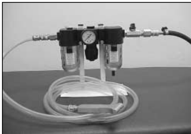
Figure 1: Compressed air massage unit consisting of two reservoir tanks, a regulator valve and inflow and outflow tubing.
