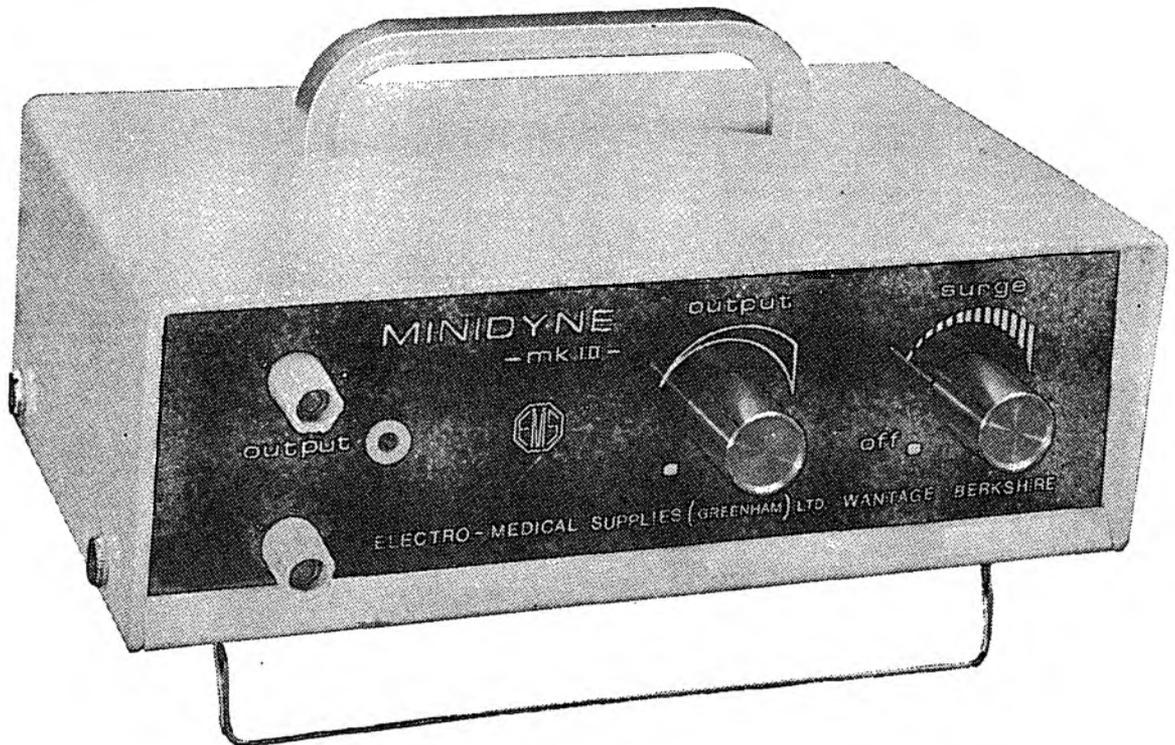
Representing another advance in the evolution of the Minidyne, the Mark III version incorporates printed circuits which reduce the size but also enhance the reliability; continuing features are
